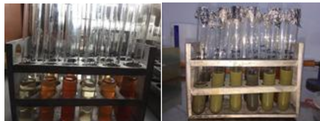
Fig 7: Green synthesis of silver nanoparticles using the aqueous extract of Syzygium aromaticum (Clove)
