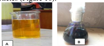
Figure 1. A.10mM FeCl 3 and B. Iron nanoparticles
