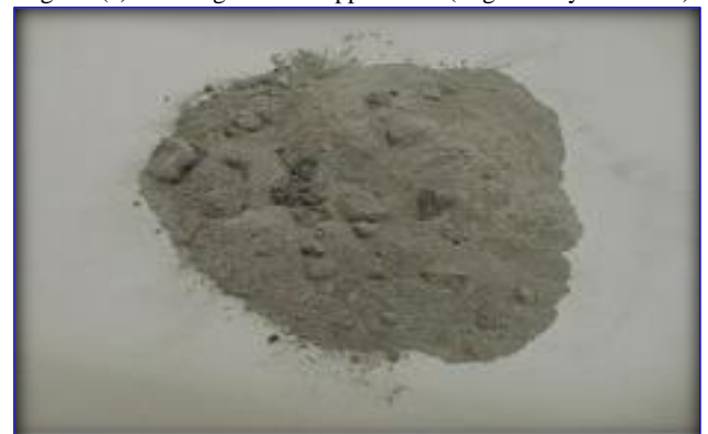
Fig. 11 (b). Completely deoxidised LF slag white in appearance
