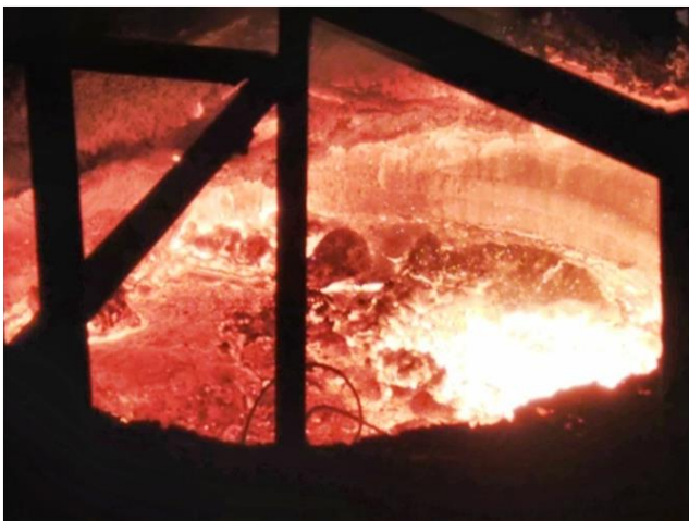
Figure 4. Crusty ladle top slag at Ladle Furnace
