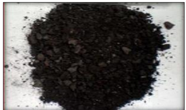
Fig. 11 (a). LF Slag black in appearance (Higher Oxy Potential)
