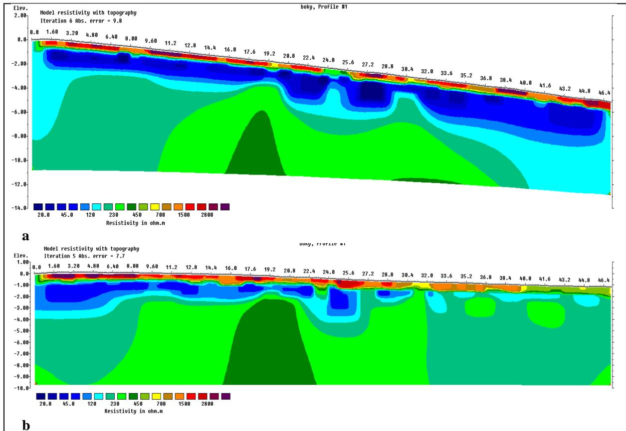
Figure 7: Soil electrical resistivity (Ohm. m) images at plot Budca-Boky; 0 m position is located at edge of the mud pit where animals use it for cooling; the highest animals disturbance appears at first 3 m, and then gradually disappear when we are getting farther from the center (mud pit); (a) electrical resistivity section from the edge of mud pit along the slope and (b) line from the edge along non-slope section.
