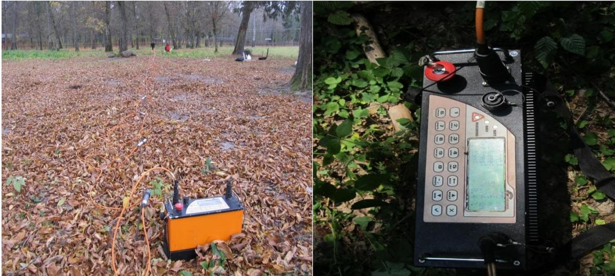
Figure 1: Electrical resistivity device (right) and electrical resistivity measurement along highly disturbed profile (left).
