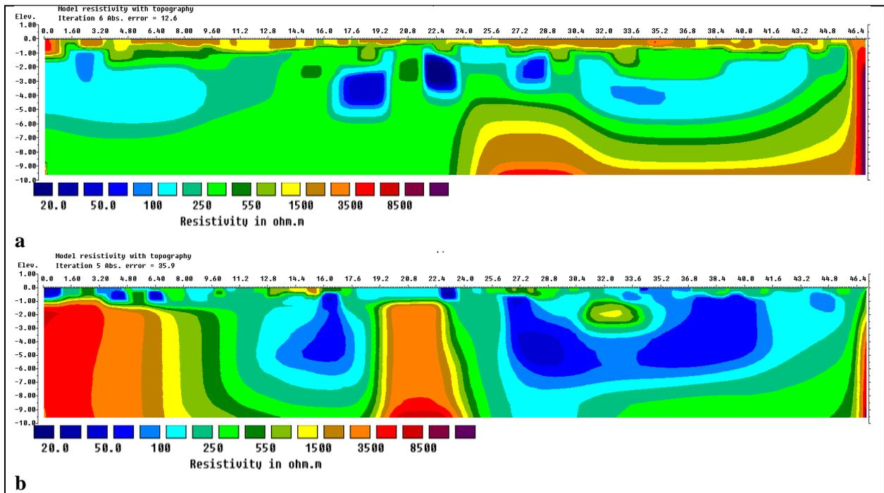
Figure 5: The visual results of soil electrical resistivity tomography (Ohm. m) images along 2 profiles at plot Topolčianky Bison Park; blue and green tones indicate low resistivity, while red, brown and yellow tones represent high resistivity; (a) is inside the Bison Park where the soil is highly disturbed by the bison, and (b) is outside the Bison Park (undisturbed plot site).
