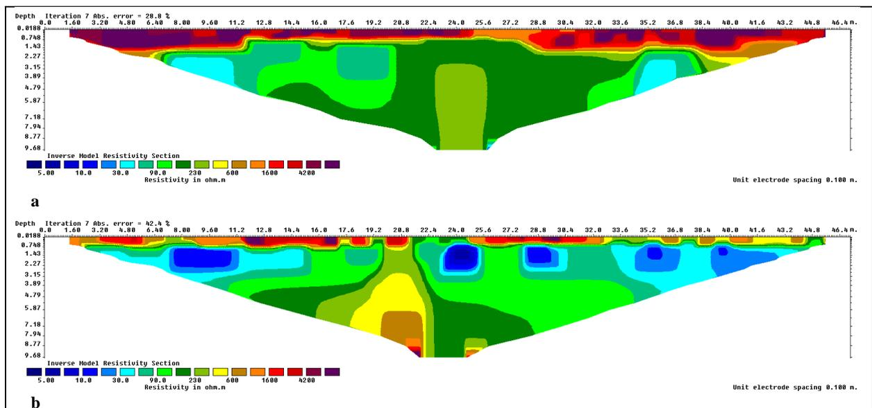
Figure 2: The visual results of soil electrical resistivity tomography (Ohm. m) along 2 profiles at plot Bialowieza Bison Park; (a) is inside the Bison Park where the soil is highly disturbed by the bison, (b) is outside the Bison Park (undisturbed plot site).
