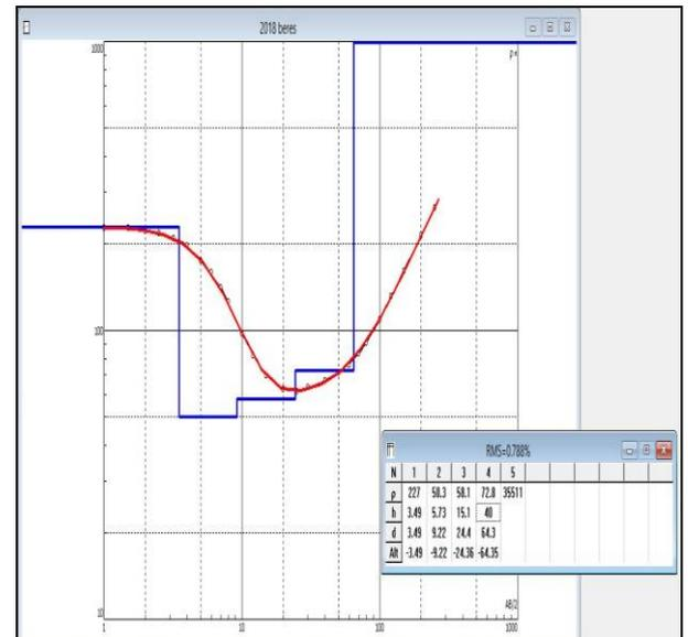
Figure 9: Geoelectric Curve for Beresiri Community
