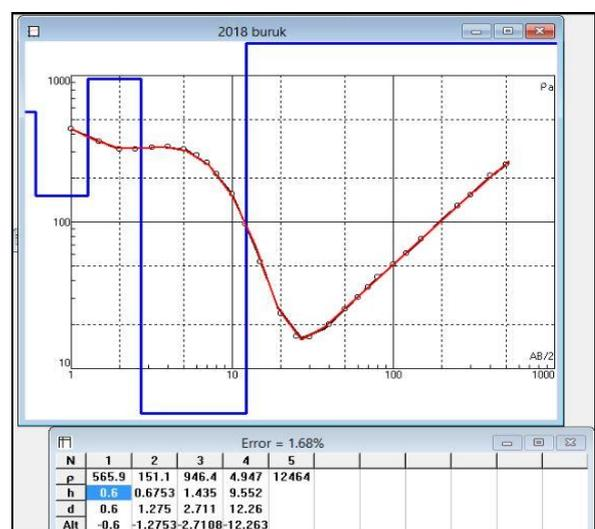
Figure 3 : Geoelectric Curve for Aru-agbalama Community
