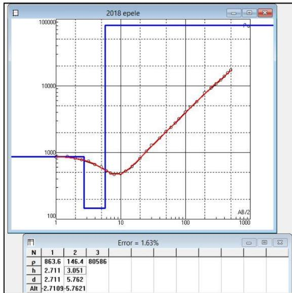
Figure 6: Geoelectric Curve for Epelema Community
