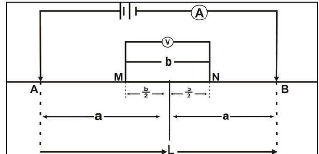
Figure 2 : Schematic Diagram for Schlumberger Array
