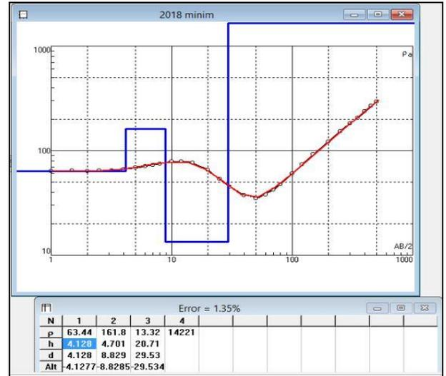
Figure 7: Geoelectric Curve for Minima Community
