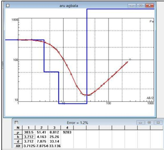
Figure 4: Geoelectric Curve for Burukiri Community
