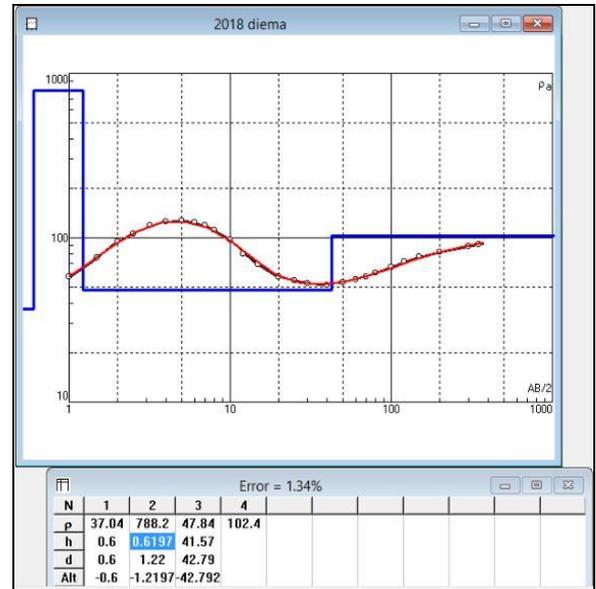
Figure 8: Geoelectric Curve for Diema Community
