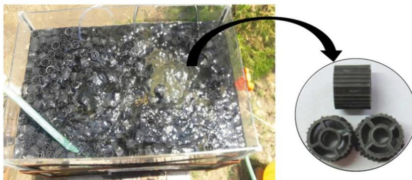
Figure 5 Real photograph of moving bed biofilm reactor and polyethylene biocarriers used for the study
