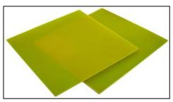
Fig 6:FR4 sheet (Epoxy Resin)
