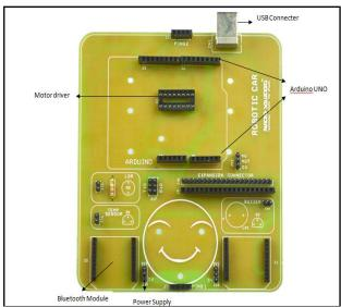
Fig 8: chassis with IC base, headers
