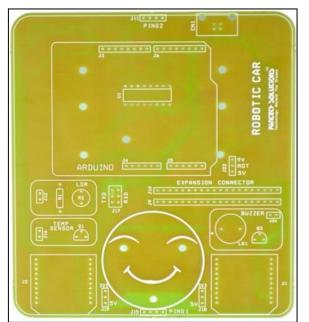
Fig 7: Printed circuit plan of robotic car
