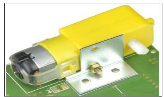
Fig 9: L-bracket attached to DC Motor
