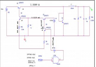
Fig.4 Switch Drive Circuit
