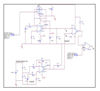
Fig6:Design of SMPS using Integrator circuit
