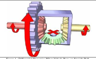
Figure 1 : Differential Dynamics When Vehicle Runs on Straight Path.
