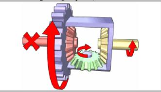
Figure 2 : Differential Dynamics When Vehicle Takes Turn.
