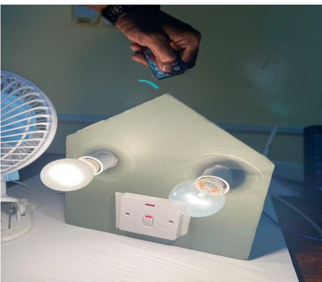
Figure 9. 60W lamp load 2 is ON/OFF.
