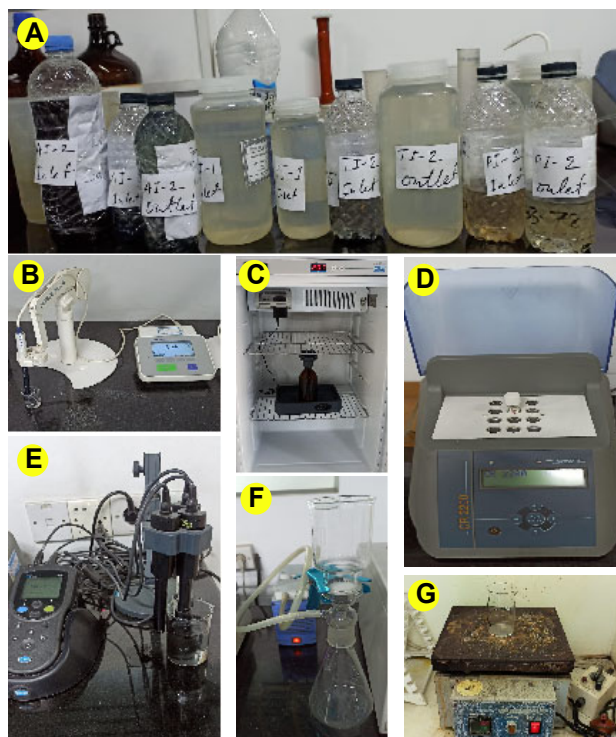
Figure 2. (A) Wastewater samples, (B) Mettler Toledo pH meter, (C) Incubator, (D) COD reactor, (E) DO meter, (F) Filtration apparatus, (G) Hot plate.
